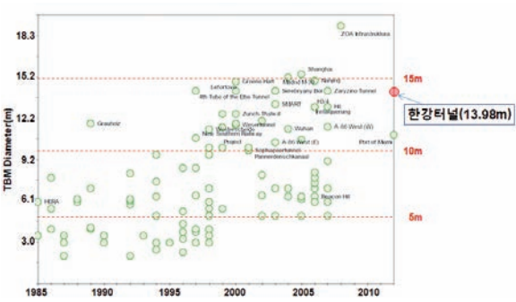
[그림 2] Increasing TBM diameters during 1985–2012
